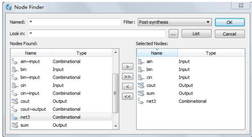
Figure: The addition of the simulation testing signal net3
