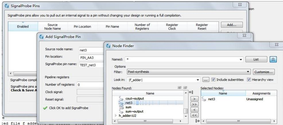
Figure: Setting the probe signal net3 in the SignalProbe dialog box
