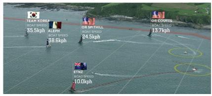
The CNS-5000 precisely determines the exact position, orientation, and movement of the America's Cup catamarans. It overlays that data along with computed distances and laylines to the marks on the race course onto video being shot from helicopters also equipped with the CNS-5000. This is all accomplished in real time for live television coverage.
