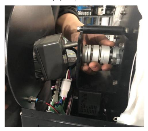
5、拆掉连轴放好 Remove the shaft and put it in place
