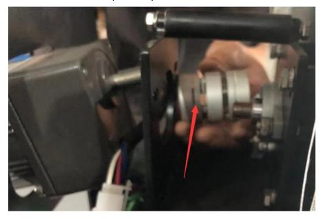
6、拧松后轴承与锅炉后轴上连接的螺丝(利用 2mm 内六角逆时针旋转) Loosen the screw connecting the rear bearing to the boiler rear shaft ( Use 2mm hexagon counterclockwise rotation)
