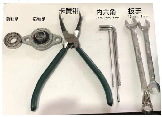
2、拆卸收集桶和门板(门板用内六角把两边的螺丝逆时针旋转拆掉即可) Remove collection bucket and drum cover(use inner hexagon screw on both sides of the counterclockwise rotation can be removed
