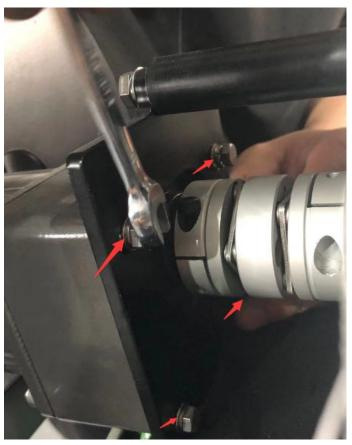
4、电机稍微轻轻往后拉一点,固定住不往下掉(注意连接线) Pulled back the motor slightly to keep it in place
