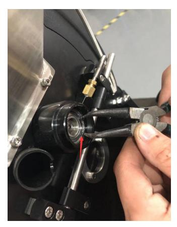
11、把锅炉后轴先往后拔再往前压,前轴承就会凸出来,这时,就可以对前轴承进行更换 The rear shaft of the boiler is pulled back and pressed forward. The front bearing will protrude. At this time, the front bearing can be replaced
