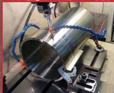
Titanium 787 landing gear torque tube in the EDM machine installing defects. Boeing will use this to calibrate instruments used for aircraft
