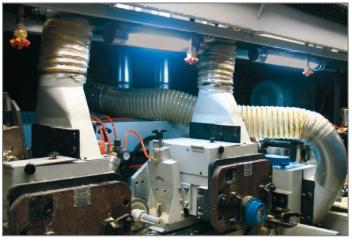
Firefly's PlanerGuard system detects sparks or incipient fire at a very early stage. The PlanerGuard system can be designed in a cost-efficient way due to the compact design of the moulder. Water mist will extinguish quickly and efficiently, even in these closed areas. Water mist also ensures that your moulder isn't damaged by water.
