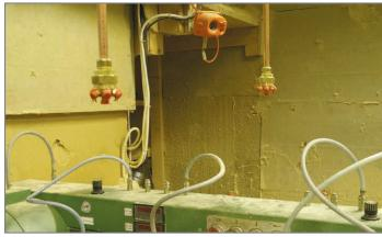
Firefly's PlanerGuard monitors this type of machine by using flame detectors monitoring the open area. It is important that extinguishing can take place even in closed areas of the planer. This is especially true for open planers. Water mist will extinguish fire quickly and efficiently, even in these closed areas. Water mist also ensures that your planer isn't damaged by water.
