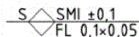
Figure 6 — Example of an indication of parting surface with specific type of parting surface, permissible mismatch and flash
