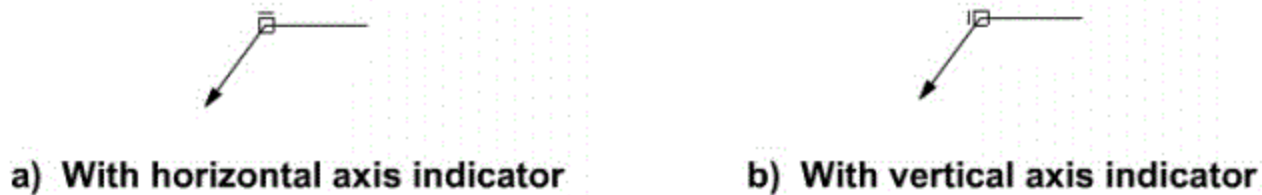
Figure 48 — Graphical symbol for indication of global all about condition used on leader and reference lines
