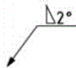
Figure 62 — Inclination symbol used with leader and reference lines
