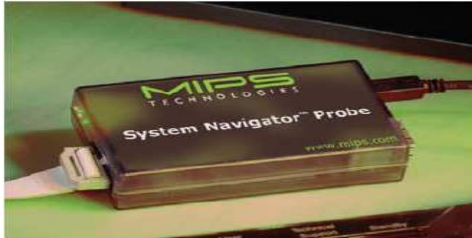
The System Navigator probe host software runs on a Windows® XP or Linux PC over a USB2.0 or 10/100 Ethernet host connection. It provides a source-level debug solution with PDtrace™ (Program and Data Trace) and complex breakpoint support when used with the MIPS Navigator™ ICS product.
