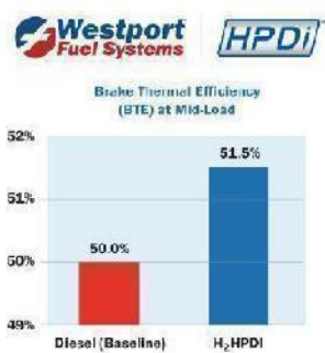
The engine test results from the Scania 13-Litre CE51 platform running with Westport's H 2 HPDI fuel system demonstrates even higher efficiency than the already super-efficient diesel engine.
