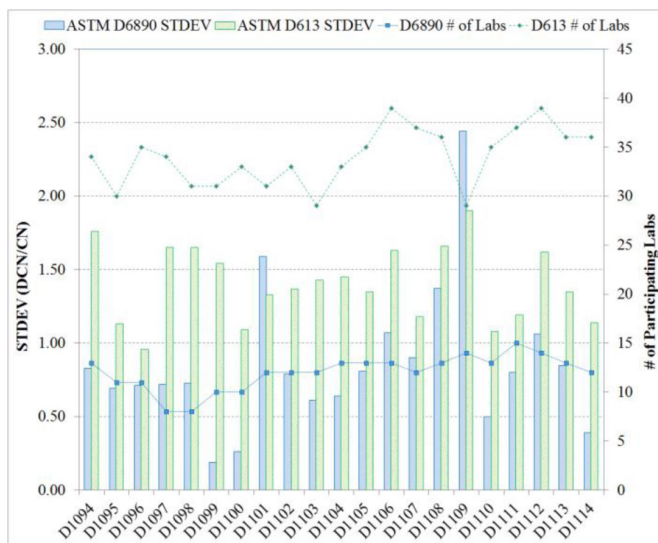
Figure 5. Number of Labs and Standard Deviations for the ASTM NEG Program (Data from January 2015 to September 2016)
