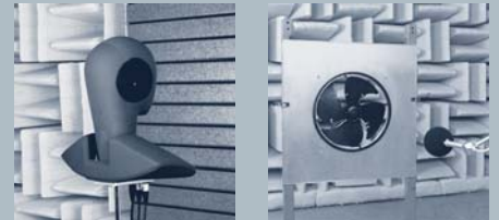
Room for precision noise measuring
