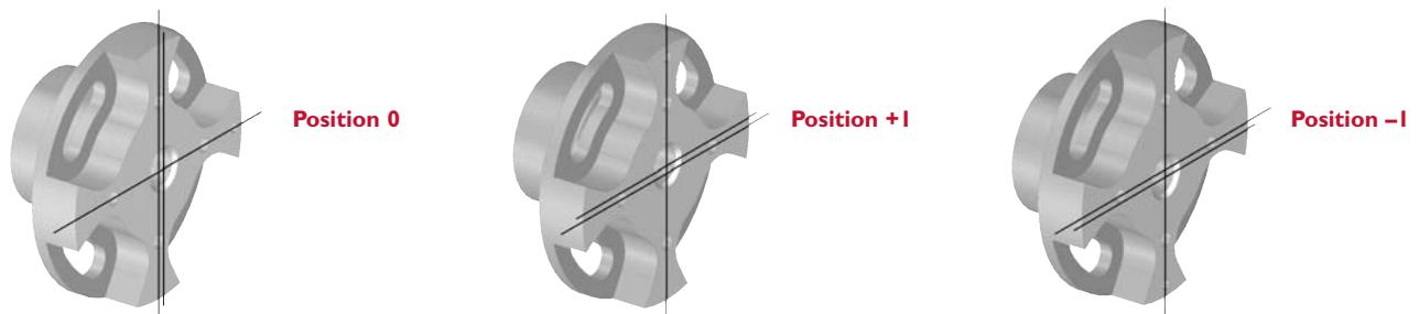
Eccentric mounting flanges KEP together with centric rollers VR..B fulfil the same function as eccentric rollers VR..A. If a roller is located in its zero position, the gear teeth backlash will be the standard value of 0.05mm flank clearance.
