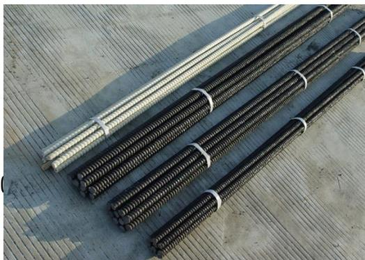
图 5FRP(Fiber Reinforced Plastics )筋
