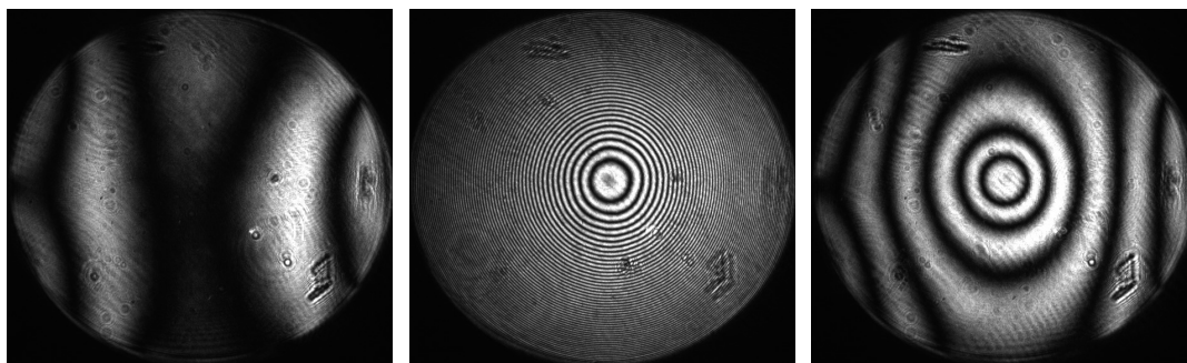
Figure 2: Test of the mirror (left to right): zero voltage applied, maximum voltage applied to all actuators, voltage applied to the central actuator. The patterns are obtained with Twyman-Green Interferometer at \lambda = 633 \text{ nm}
