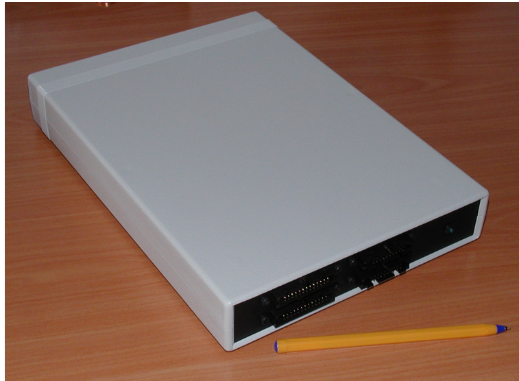
Figure 3: 40 channel high-voltage amplifier unit.
