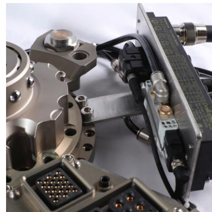
**R****机器人侧基础单元****T****工具侧基础单元**
