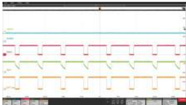
Ch1 = V_{(SUPPLY)} Ch2 = V_{(DIAGEN)} Ch3 = V_{(PWM1)} Ch4 = V_{(OUT1)} Ch5 = I_{(OUT\_Tot)} Figure 8-5. 200-Hz PWM Dimming at 80% Duty Cycle
