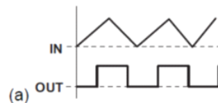
Figure 7. Schmitt Trigger Curves
