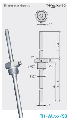
Immersion sleeve, stainless steel V4A (1.4571) with neck tube
