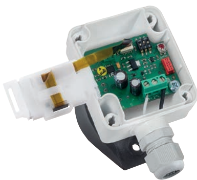
TM 65 with display and quick-locking screws (IP 67)
