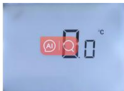
TEMP lower limit Threshold
