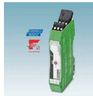
设备耦合器，用于FOUNDATION Fieldbus 和PROFIBUS PA 页512
