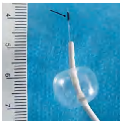
Fig. 1 The tip of the laser fiber was packaged with a radiopaque ring mark (black arrow).
