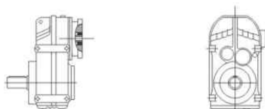
F(FF, FA, FAF, FAZ)..Y.. 电机用户自配或配特殊电机时需加联接法兰 When equipping the user's motor or the special one, the flange is required to be connected
