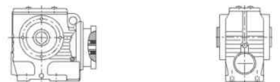
SA(S, SF, SAF, SAZ)S..R.. 电机用户自配或配特殊电机时需加联接法兰 When equipping the user's motor or the special one, the flange is required to be connected
