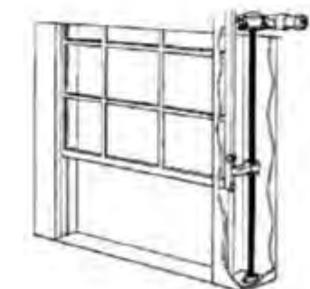
大型窗户(门)自动开关 Automatic switch on large windows (doors)
