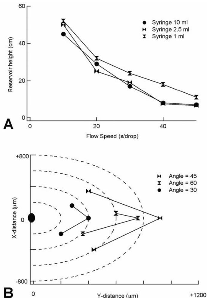
**Figure 4.** Effect of reservoir height and pipette angle. (A) Effect of reservoir height (cm) on flow rate (seconds per drop) for 10 ml, 2.5 ml and 1 ml syringes. (B) Effect of pipette angle on territory under control. Test conditions: reservoir height = 40 cm, flow rate = 18 s/drop, tip I.D. = 100  $\mu\text{m}$ . The recording pipette was placed at various distances up to 1200  $\mu\text{m}$  from the puffing tip, which was fixed at 0,0, indicated by the small grey circle on the x-axis.
