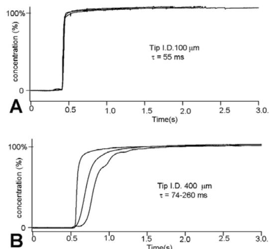
**Figure 2.** Consistency of drug-delivery kinetics among different tubes. Superimposed traces from a sensing electrode to puffs from each of the seven tubes in one puffing pipette. Note that the puffing tip with 100  $\mu\text{m}$  tip diameter evoked fast and consistent responses (A), while in a 400  $\mu\text{m}$  tip, different tubes evoked significantly different response kinetics (B).
