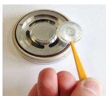
Brake wear particles are collected in the impactor of the HR-ELPI®+ in 14 separate size fractions for later microscopical or chemical analysis
