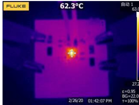
Figure 24. Thermal Image (VIN=24V, VO=5V, 0.6A)
