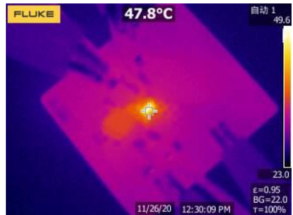
Figure 23. Thermal, 24VIN, 5Vout, 0.6A
