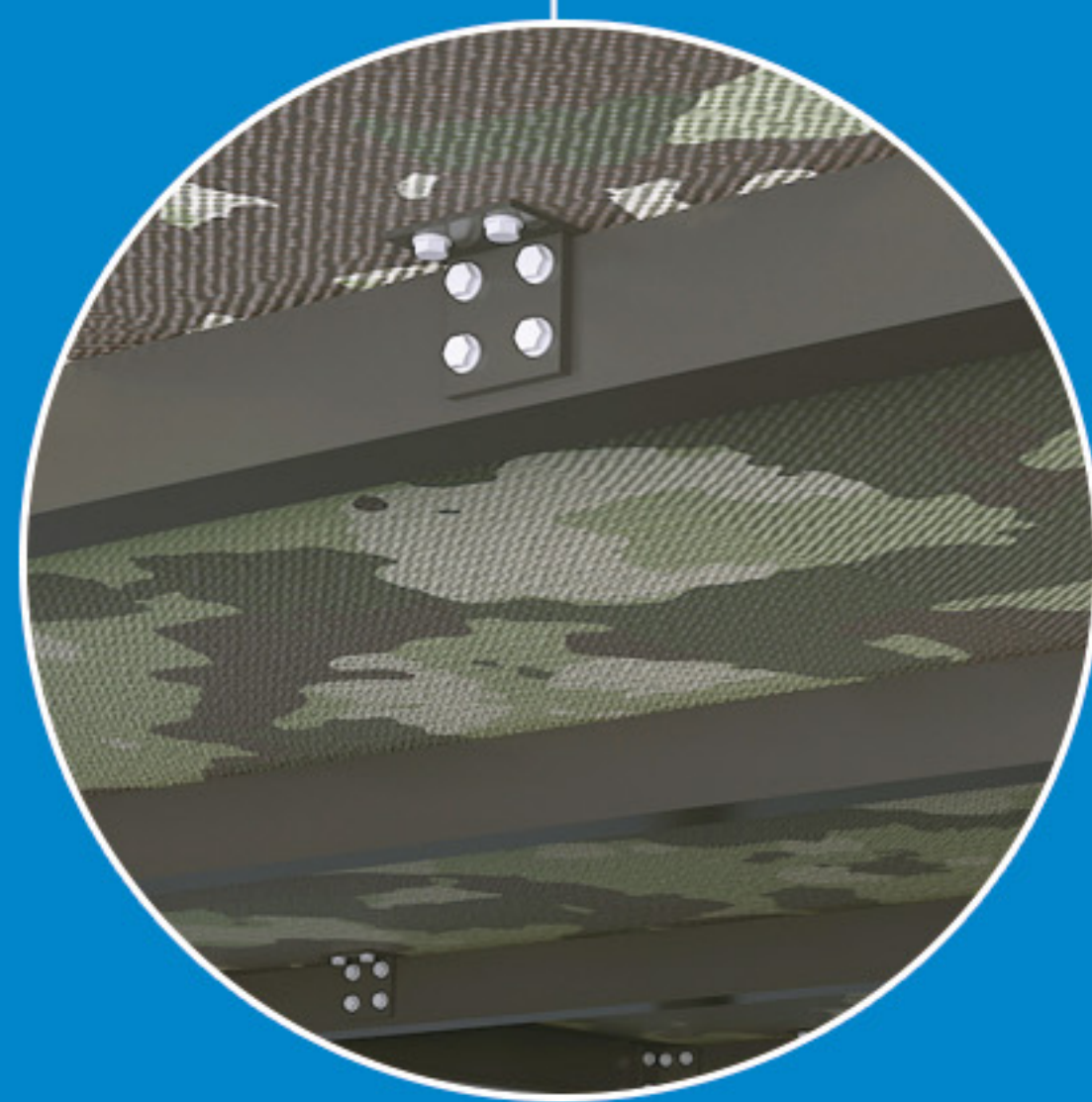
Floor connects to U-steel base by bolts
