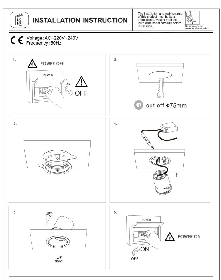
1 Disconnect the voltage from the system before performing the installation.
