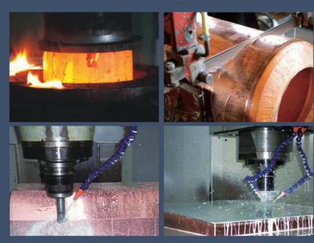
**SMMC** copper moulds manufacturing plant is a completely integrated plant with capacity more than 35,000 pcs per year including copper melting and casting units, hot extrusion, hot and cold drawing machines, machining equipments, electric plating units and various inspection equipments. The fact of with the entire manufacturing process under our direct control can ensure our product quality also the delivery time.
