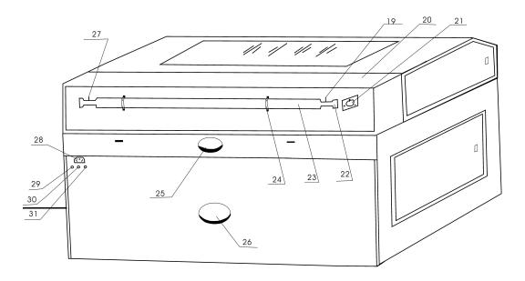
Figure 2: Sketch map of the laser engraving machine's back side
